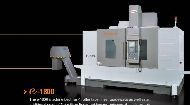
additional span of 2 auxiliary linear guideways between, that allows this machine to handle heavy loading and maintain outstanding stability.
